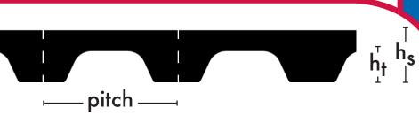
For belt part number, measure width, pitch and length (mm). Example: 50-AT10-1000= 50mm wide; 10mm pitch; 1000mm long
