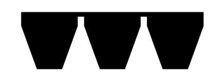
Wedge or Thunder Wedge V-Belts bound together with a fabric tie band. For belt part number, indicate number of ribs and Wedge V-Belt part number. Example: 4/8V3150= 4 rib 8V3150
